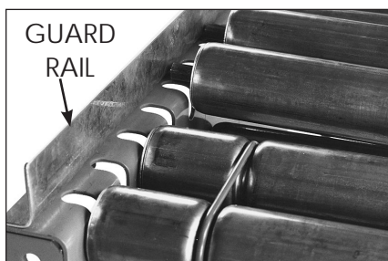
WHEN GUARD RAIL IS ADDED, DO NOT COVER POP OUT SLOTS IN CONVEYOR FRAME*
