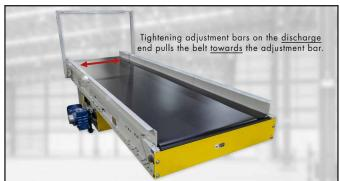
Tightening adjustment bars on the discharge end pulls the belt towards the adjustment bar.
