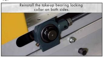
Reinstall the take-up bearing locking collar on both sides.
