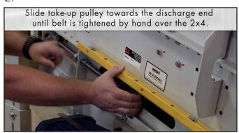
Slide a take-up pulley towards the discharge & until belt is tightened by hand over the 2x4.
