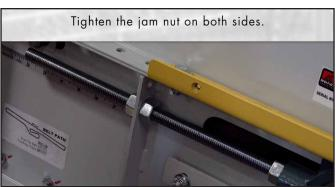
Tighten the jam nut on both sides.
