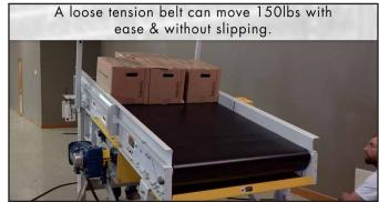
A loose tension belt can move 150lbs with ease & without slipping.
