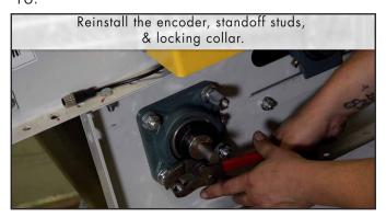
Reinstall encoder, standoff studs, & locking collar.
