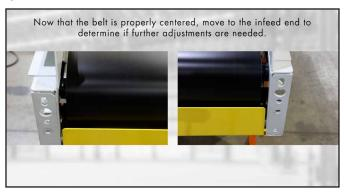
Now that the belt is properly centered, move to the infeed end to determine if further adjustments are needed.
