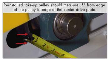
Reinstalled take-up pulley should measure .5" from edge of the pulley to ede of the center drive plate. 16.
