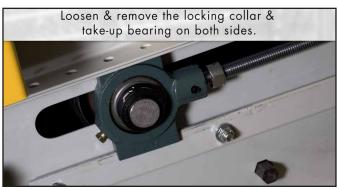
Loosen & remove the locking collar and take-up bearing on both sides.
