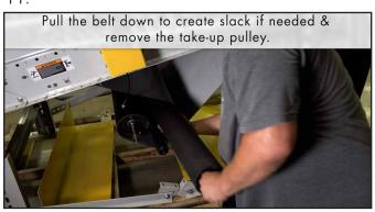
Pull the belt down to create slack if needed & remove the take-up pulley.
