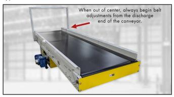
When out of center, always begin belt adjustments from the discharge end of the conveyor.
