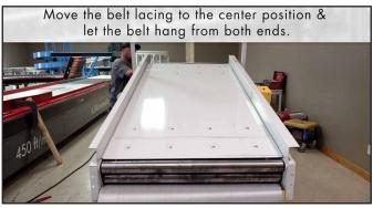
Move the belt lacing to the center position & let the belt hand from both sides.
