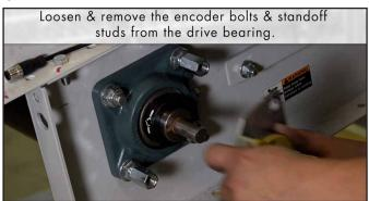
Loosen & remove the encoder bolts and standoff studs from the drive bearing.
