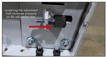
Loosening the adjustment bolt increases pressure on the adjustment bar.
