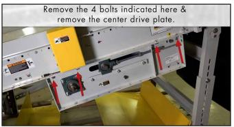
Remove thr 4 bolts indicated here & remove the center drive plate.
