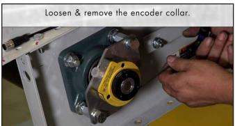
Loosen & remove the encoder collar.
