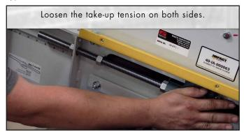
Loosen the take-up tension on both sides.
