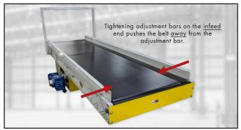
Tightening adjustment bars on the infeed end pushes the belt away from the adjustment bar.
