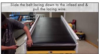
Slide the belt lacing down to the infeed end & pull the lacing wire.
