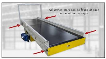
Ajustment bars can be found on each corner of the conveyor.
