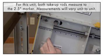
For this unit, both take-up rods measure to the 2.5" marker. Measurements will vary unit to unit.
