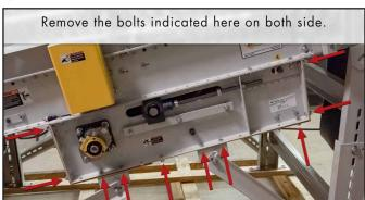
Remove the bolts indicated here on both sides.
