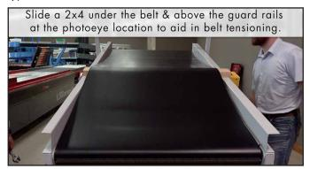
Slide a 2x4 under the belt & above the guard rails at the photoeye location to aid in belt tensioning.
