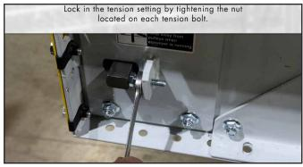
Lock in the tension setting by tightening the nut located on each tension bolt.
