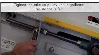
Tighten the take-up pulley unitl significant resistance is felt.
