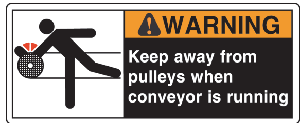
ABOVE: Label placed near all pulleys (center drives, end drives, tail pulleys)
