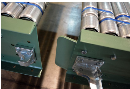
Step 1 Align the discharge end of the 1st section with the infeed end of the 2nd section.
